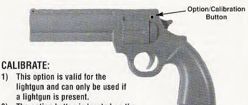
The option button is located on the upper left side of the lightgun. Refer to diagram of lightgun.
